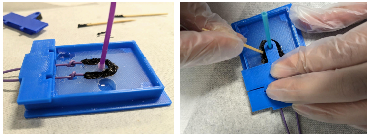
Left: Grease slightly higher than the silicone Right: Using a toothpick to push wires under the grease
