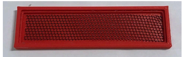
Base mold with strip of screen mesh fitted to the inside
