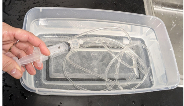
Filling syringe and tubing with water
