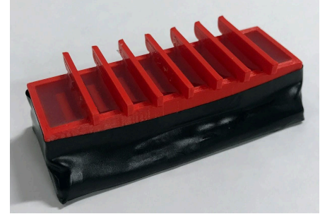
Tabs place in mold filled with uncured silicone
