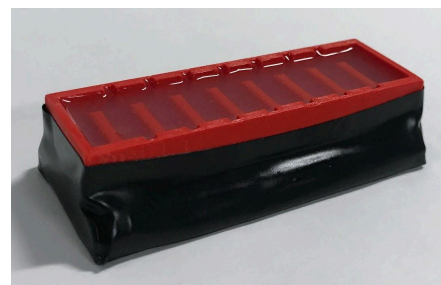
Taped mold filled with uncured silicone rubber
