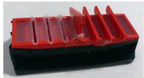
Tabs being removed from cured silicone
