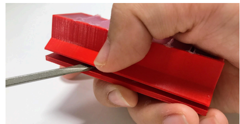
Prying apart the mold pieces using a flat blade screwdriver
