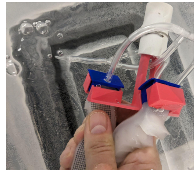
Squeezing air bubbles out of gripper underwater
