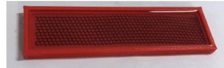
Base mold partially filled with uncured silicone
